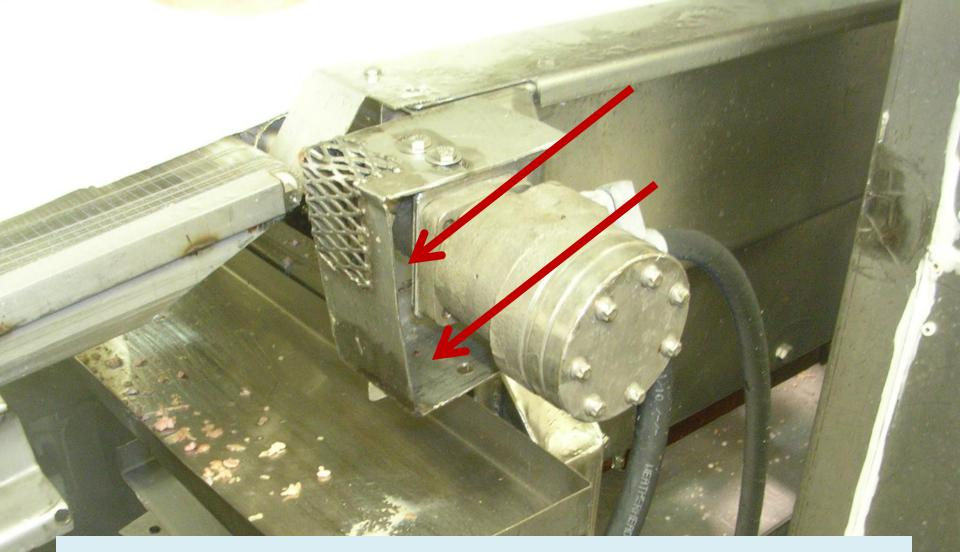
Guards not adjusted properly to completely cover rotating parts
