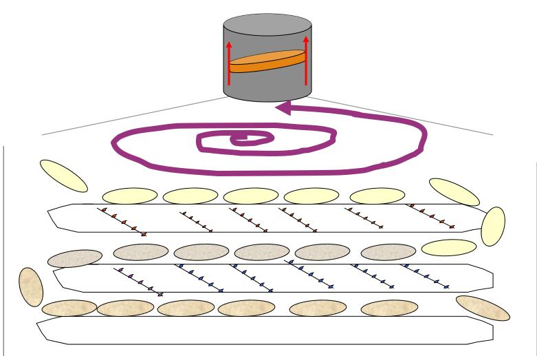
Negative air pressure increases humidity in the baking chamber as well as increases the latent heat (convective and radiant). Causes pillowing and increases surface moisture
