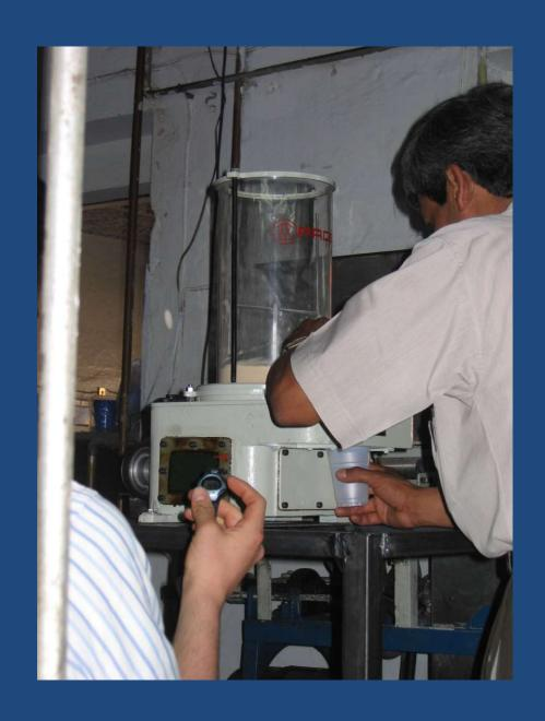
Adjust dosifier flow rate to match mill flow rate (I g premix/Kg masa)
